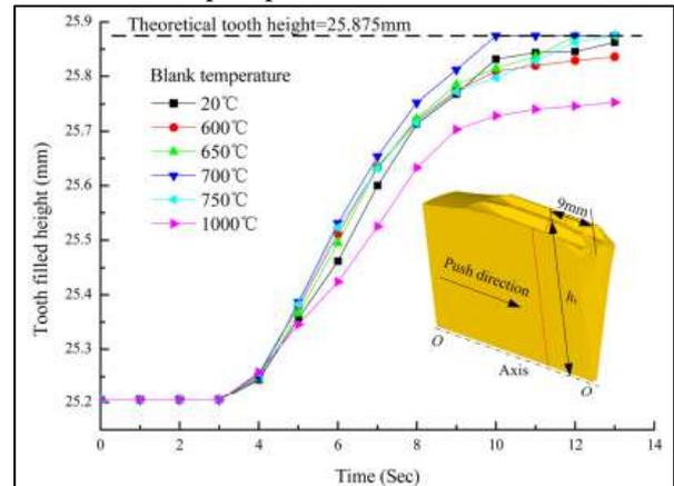
Fig. 4: Comparison on tooth-filled height under different deformation temperatures [14]
