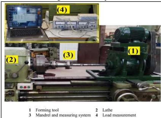
Fig. 10: Test rig components of forming process. [16]
