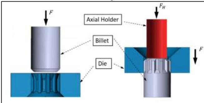
Fig. 6: Spline-forming process [15]
