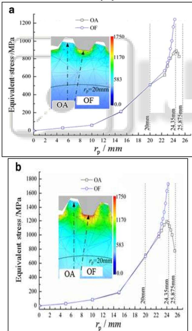
Fig. 3: The equivalent stress distribution of the spline shaft: a preformation area and b correction formation area [13]
