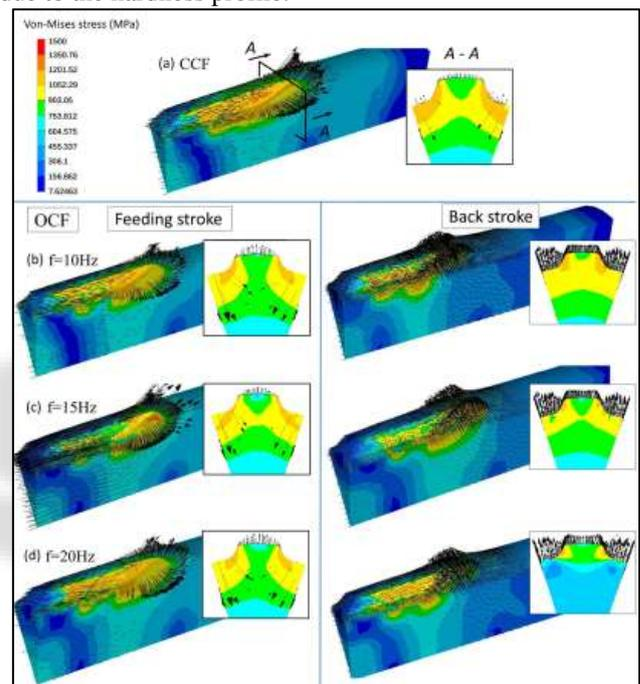
Fig. 1: Von-Mises stress and velocity distribution of the workpiece in different condition [12]
