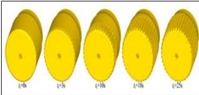
Fig. 2: 5 Diagram of formation process of the spline shaft by FEM [13]
