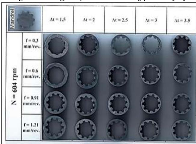
Fig. 11: (a) The cross section of internally-spline sleeves at various axial feed and cross in-feed. (b) The internally-spline sleeves at various cross in-feed [16]
