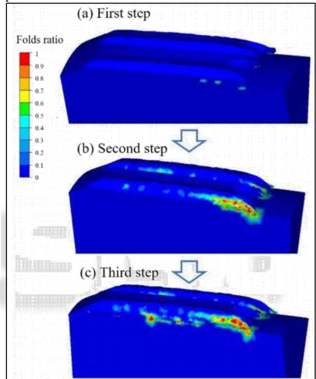
Fig. 9: Distribution of folds at the first step (a), second step (b) and third step (c) in the forming method of assembling dies [16]
