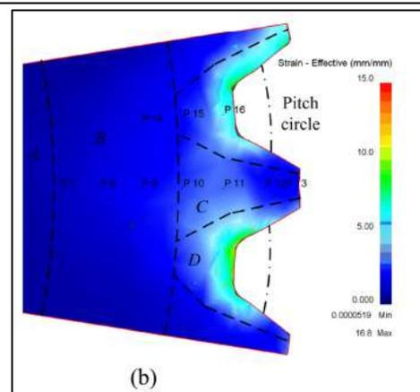
Fig. 5: Effective strain of the selected point under different radius, a the values of the effective strain and b schematic diagram of the selected points and four different deformation regions [14]
