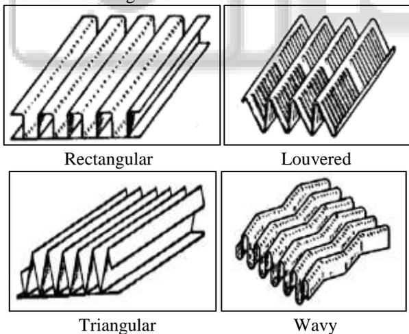
Fig. 1.3: Surface geometries of plate-fin exchanger: (A) plain rectangular fins, (B) louvered fins (C) Triangular fins (D) Wavy fins.
