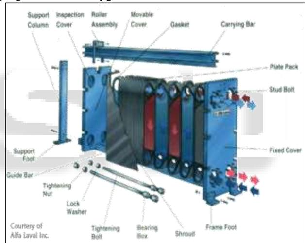
Fig. 1.4: An exploded view of a plate heat exchanger
