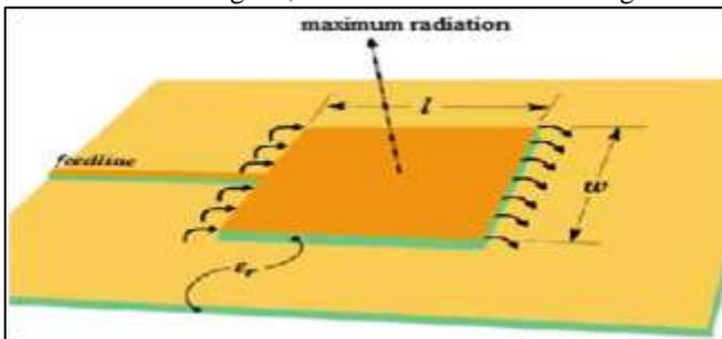
Fig. 1.1: Basic configuration of microstrip patch antenna
