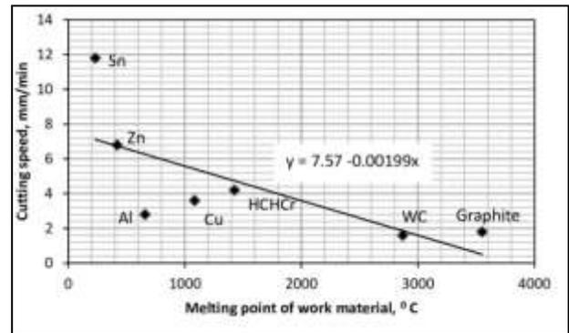
Fig. 4: Variation of cutting speed with melting point of work piece. All the experiments were carried out by cutting 10 mm x 10 mm piece of 10 mm height.
