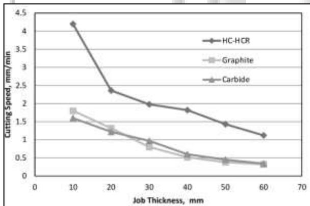
Fig. 3: Effect of cutting speed on job thickness and materials.
