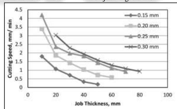
Fig. 1: Variation of cutting speed with job thickness and various diameter of wire (Job - HCHCr).
