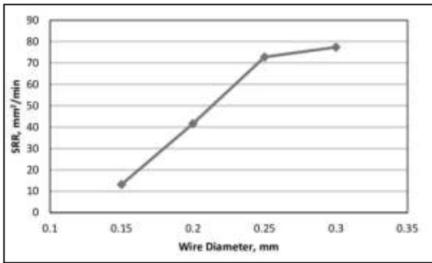
Fig. 2: Dependence of SRR with wire diameter (Job – HCHCr, Job height – 40 mm).
