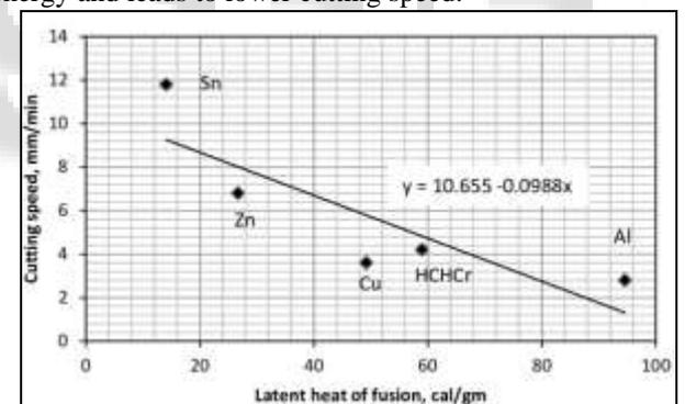
Fig. 5: Variation of cutting speed with latent heat. All the experiments were carried out by cutting 10 mm x 10 mm piece of 10 mm height.
