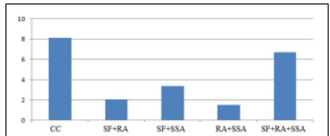
Fig. 1: Percentage of Mass Loss on Salt Resistance Test
