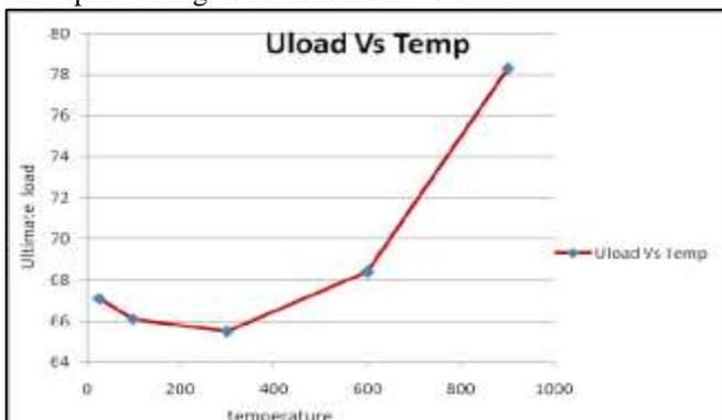
Fig. 4.1: Temperature Vs Ultimate Load
