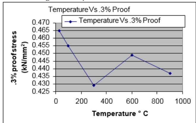
Fig. 4.9: Temperature Vs .3% Proof Stress
