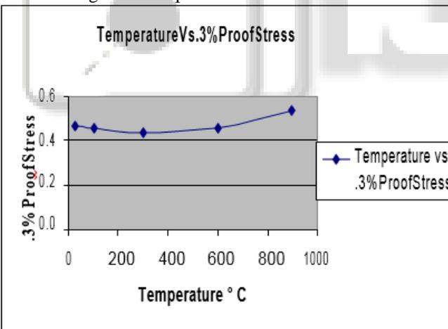
Fig. 4.4: .3% Proof Stress Vs Temperature
