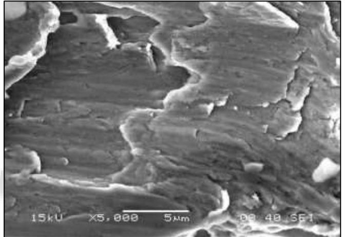
Fig. 4.14: 100° C Ordinary Cooling at Magnification of 5 Microns
