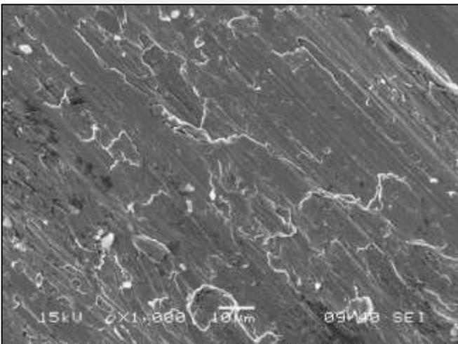
Fig. 4.18: 900° C Ordinary Cooling at Magnification of 10 Micron
