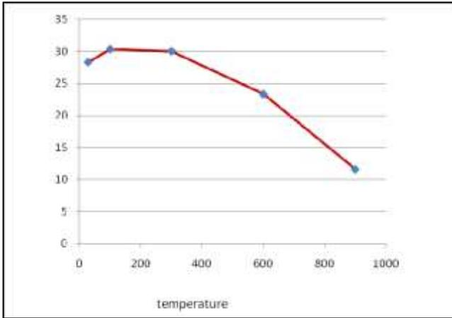
Fig. 4.2: Temperature Vs % Elongation
