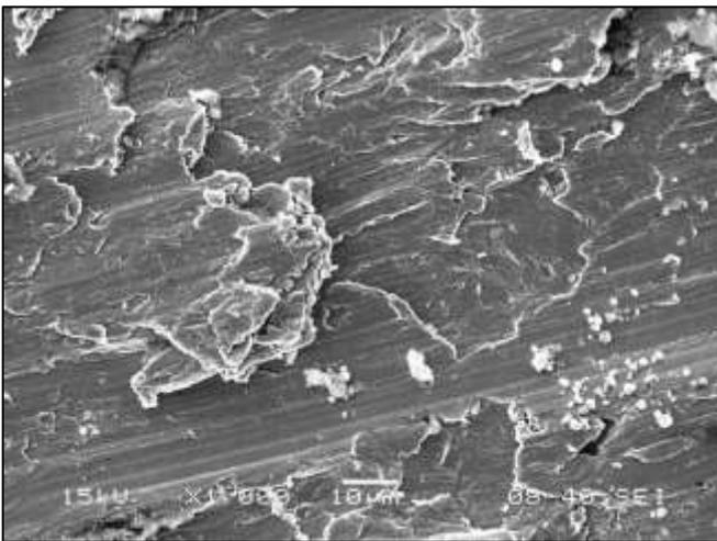
Fig. 4.17: 300° C Rapid Cooling at Magnification of 10 Microns
