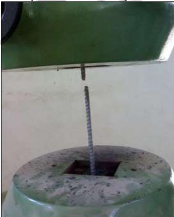
Fig. 4.12: Specimen failed on UTM.
