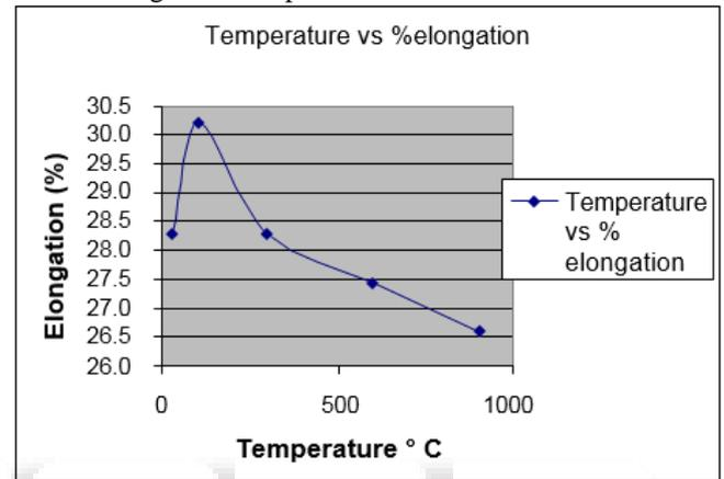
Fig. 4.7: Temperature Vs % Elongation
