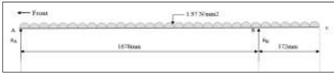
Fig. 1: simply supported beam carrying UDL
