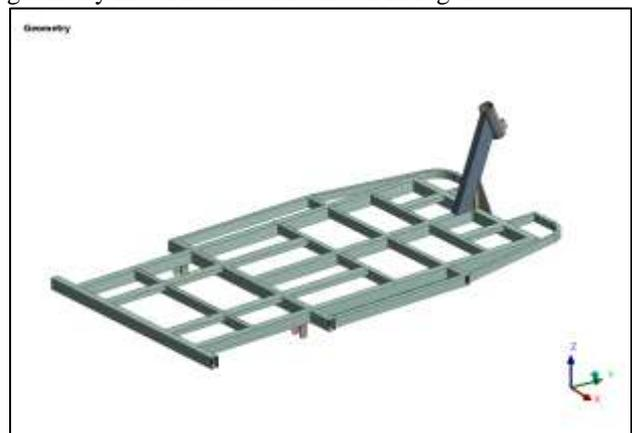
Fig 4: CAD Model of Chassis Frame
