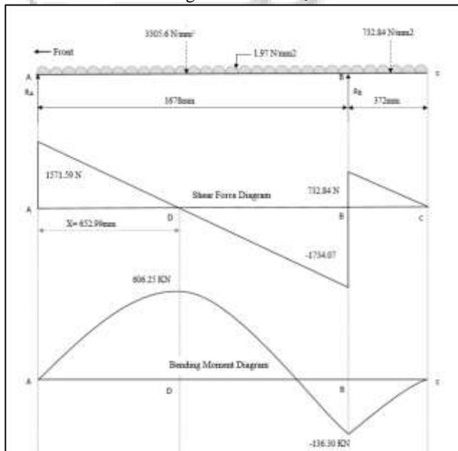
Fig. 2 Shear force and Bending Moment Diagram
