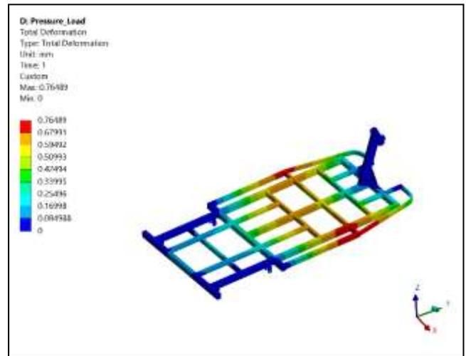
Fig. 7: Total Deformation of chassis under loading Stress: The location of maximum Von Misses stress and maximum shear stress are at bottom of mounting bracket at front of chassis which is showed in figure below. The Von Misses stress magnitude of critical point is 137.33MPa.
