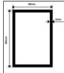
Fig. 3: Rectangular Cross Section
