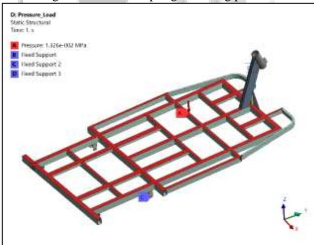
Fig. 6: Structural Load and boundary Condition for chassis frame
