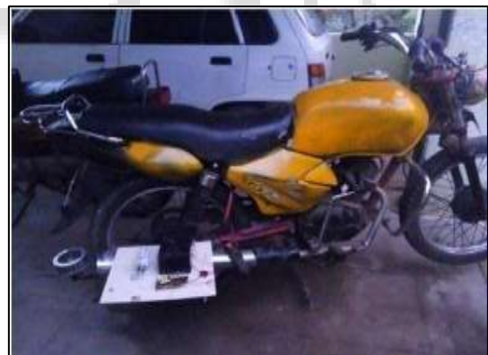
Fig. 2: model of bike using energy generation from exhaust gases
