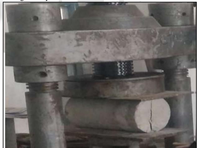
Fig. 7.4: split tensile test
