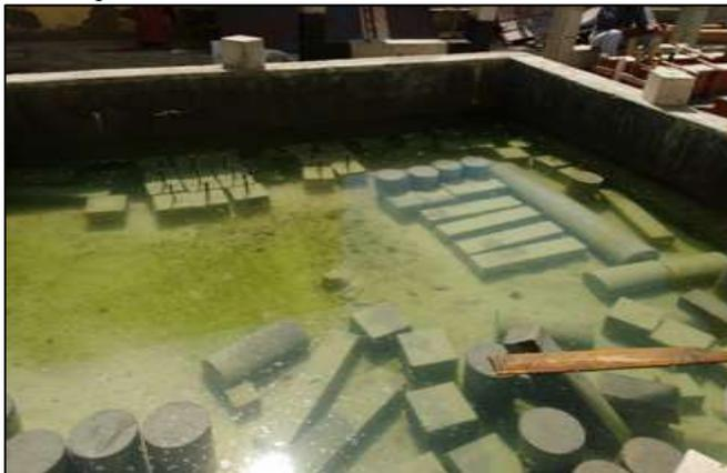
Fig. 5.2: Curing of test specimens.
