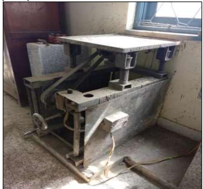
Fig. 5.1: Vibrating table
