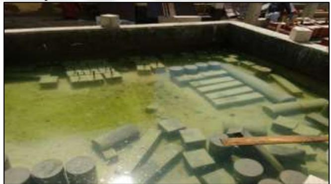
Fig. 5.2: Curing of test specimens.
