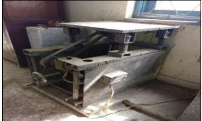
Fig. 5.1: Vibrating table
