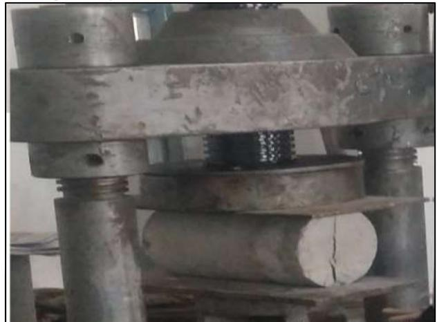
Fig. 7.4: split tensile test
