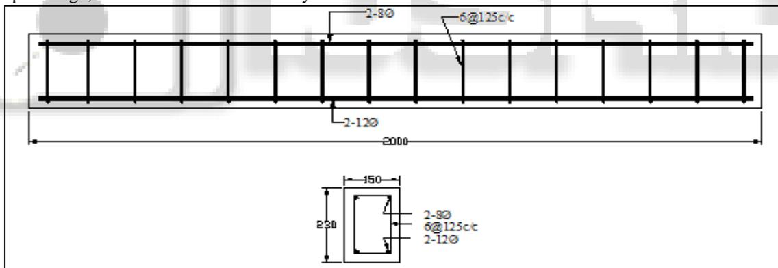
Fig. 1.1: Reinforcement details of beams
