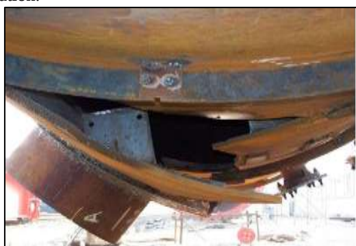
Fig. 1: Internal Pressure Failure
