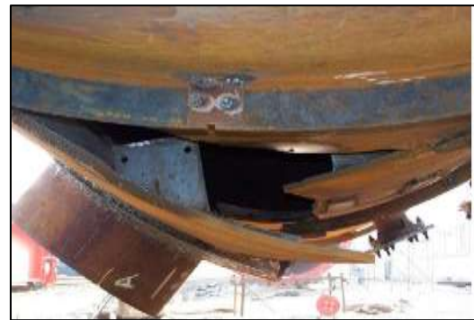
Fig. 1: Internal Pressure Failure
