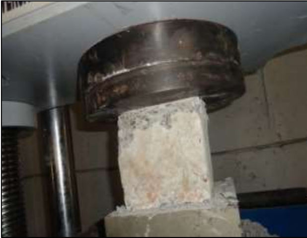
Fig. 2: Compressive Strength Test
