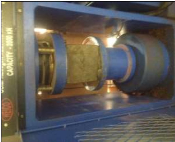
Fig. 3: Compressive Strength Test perform
