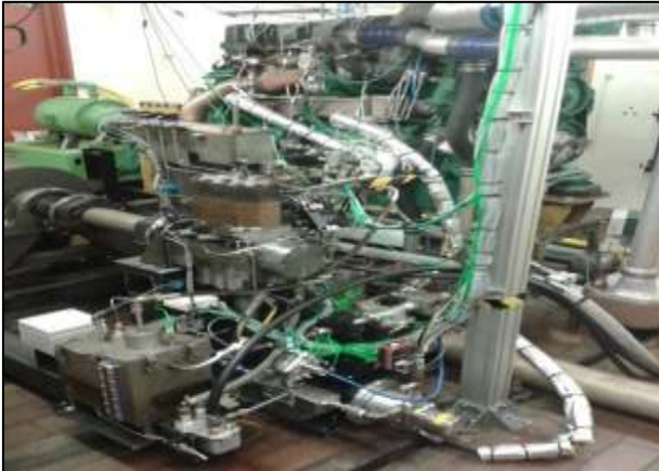
Fig. 6: Experimental setup of the heat recovery system in the engine test cell
