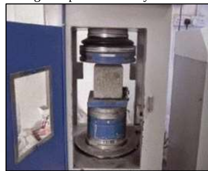
Fig. 3: Compressive Strength test on Cube
