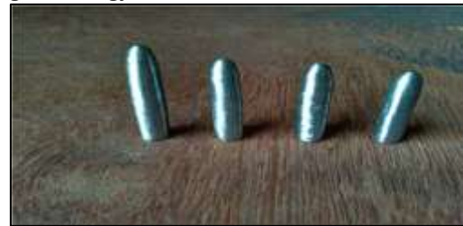
Fig. 7: Specimen Extracted From Hardfaced Plate
