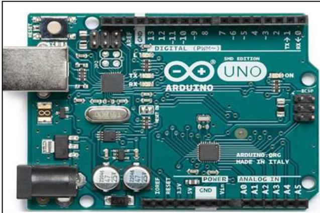
Fig. 2: Arduino Uno Micro Controller
