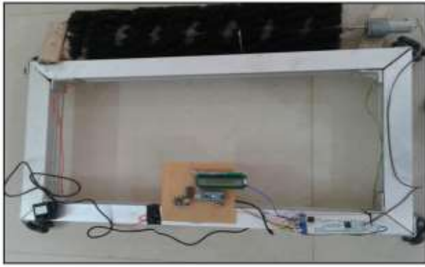
Fig. 2.2: Working model of solar panel cleaning robot using IoT
