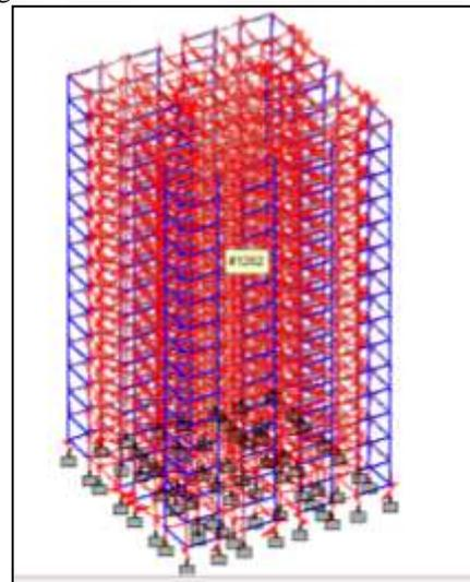
Fig. 4: BENDING MOMENT DIAGRAM
