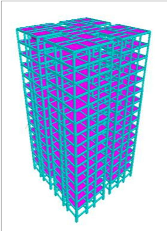
Fig. 4: 3D view of structure without shear walls
