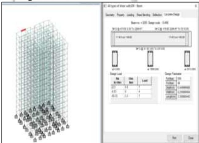
Fig. 8: REINFORCEMENT DETAILS IN BEAM NO.3255
