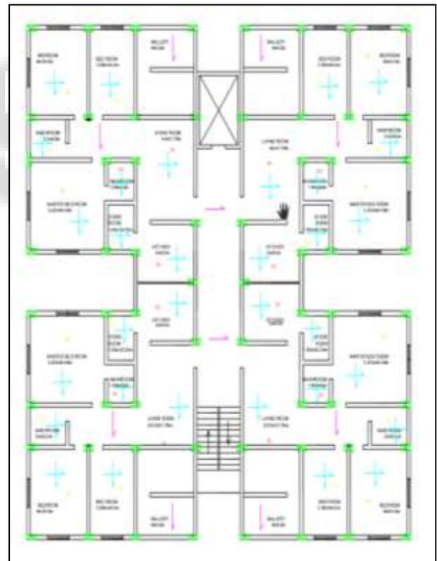
Fig. 2: 2D plan without shear walls
