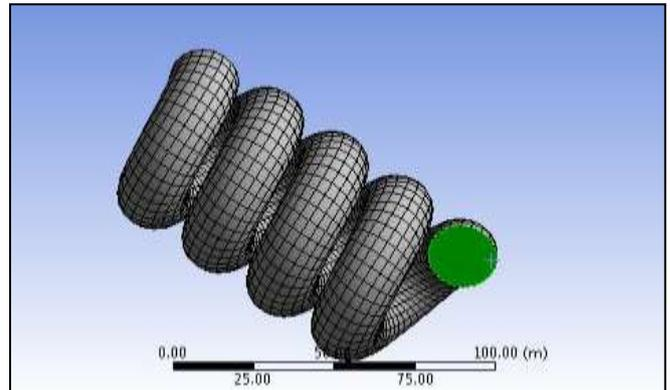
Fig. 5.3: Meshing of model
