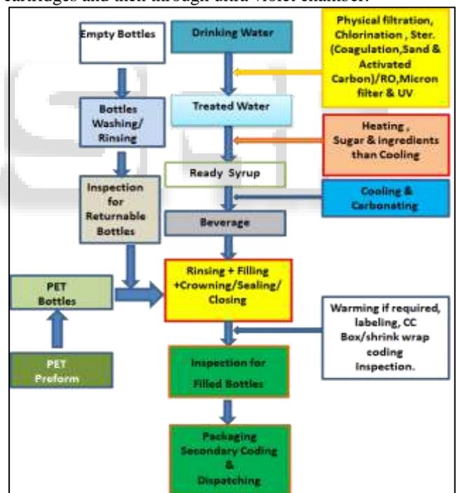
Fig.1: Flow Chart for Production Process
