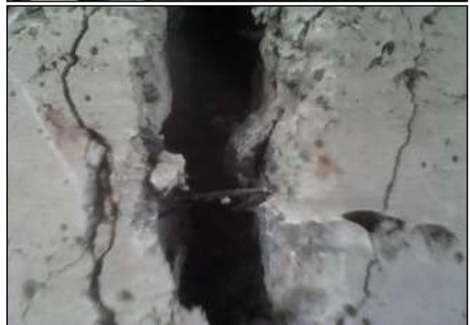
FAILURE IN SPILT TENSILE STRENGTH
