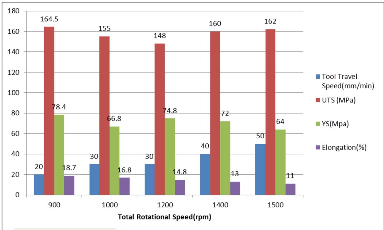
Fig. 11: Tensile Properties of Weld joint
