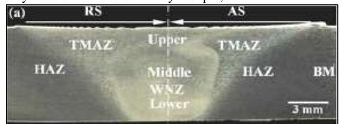
Fig. 6: Microstructure of FSW Joint
