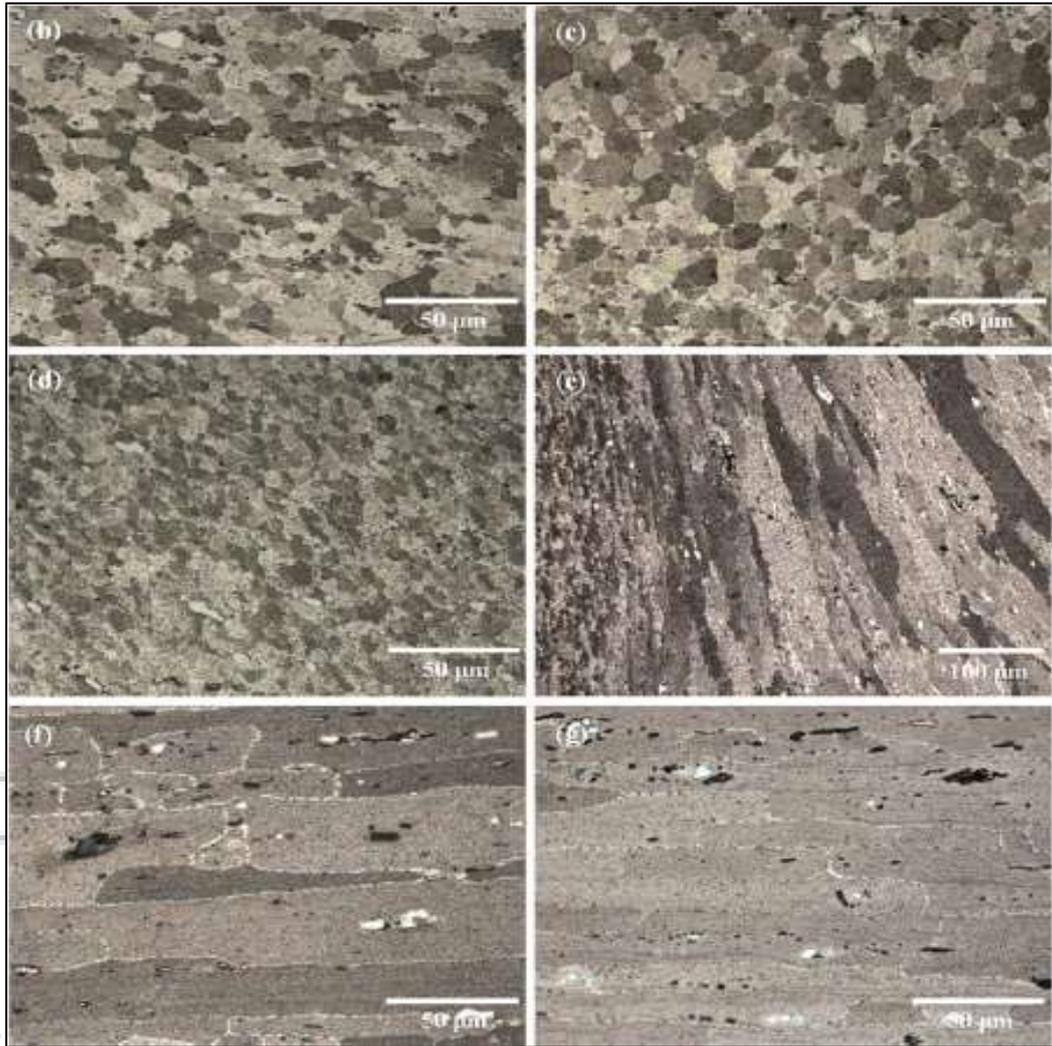
Fig. 7: a, b, c, d (Upper, middle, lower Part of WNZ), e ( TMAZ) ,f (HAZ), g (BM)
