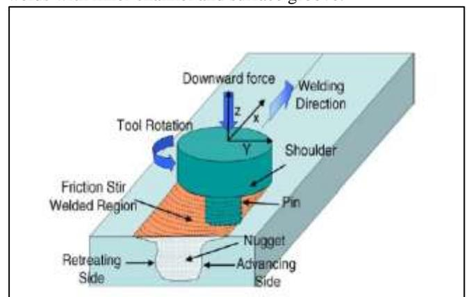
Fig. 1: Schematic Diagram of Friction stir welding Joint
