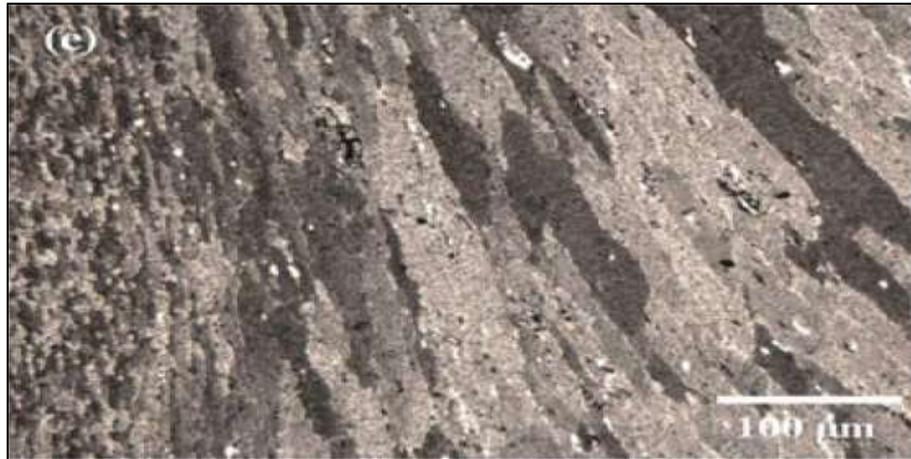
Fig. 9: Microstructure of Thermo-mechanically affected zone in aluminium 7075
