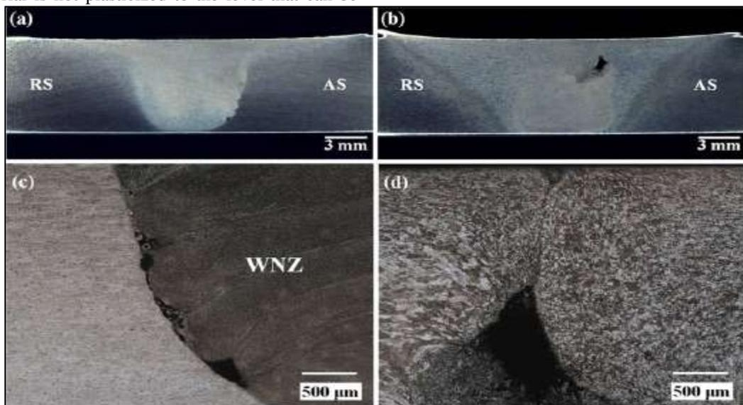
Fig. 8: Welding defects in the joint welded at different welding parameters, a. Rotational speed 1000rpm at 30mm/min, b. Rotational speed of 1200 rpm at 30mm/min, c, d Enlarged view of welding defects
