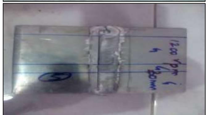
Fig. 4: Friction stir welding of Aluminium 7075
