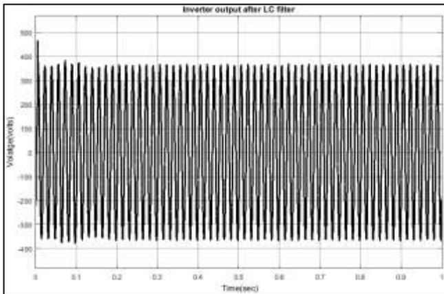
Fig. 6.22: Inverter output voltage
