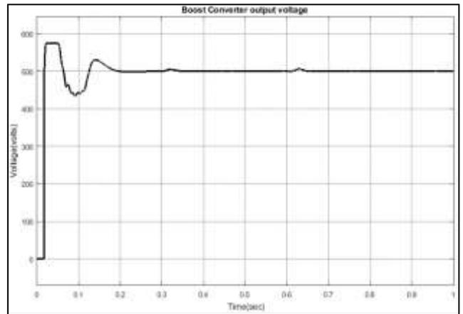
Fig. 6.18: boost converter output voltage
