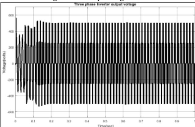
Fig. 6.17: Inverter output voltage.
