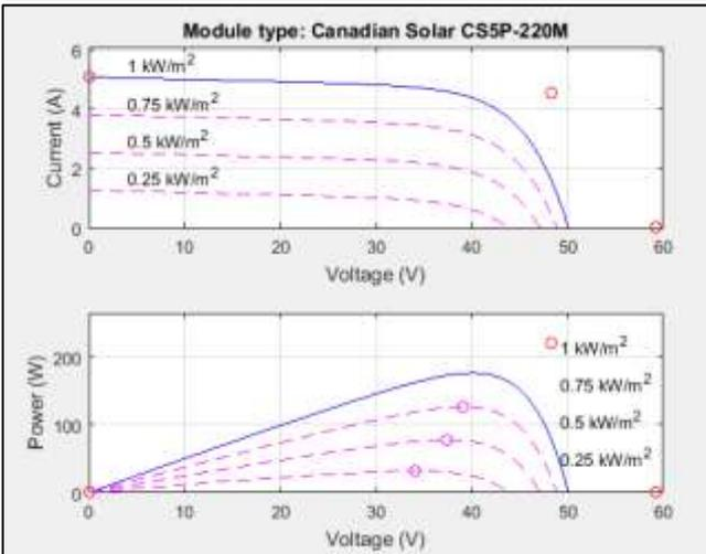
Fig. 6.8: I-V and P-V curve of solar module
