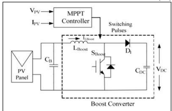
Fig. 6.3: DC-DC boost converter
