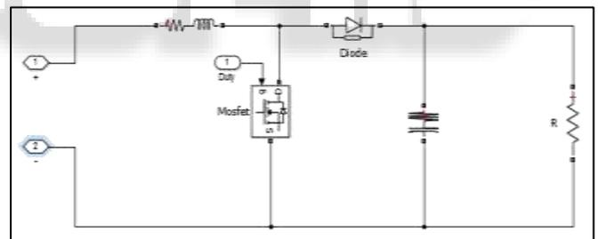
Fig. 6.12: Design of boost converter in SIMULINK
