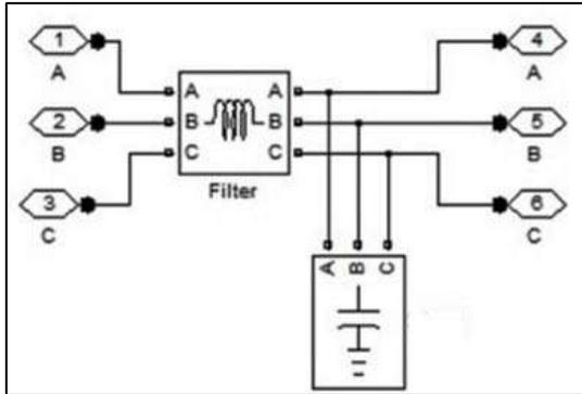
Fig. 6.4: LC low pass power filter used at the output terminals of PV inverter [12].
