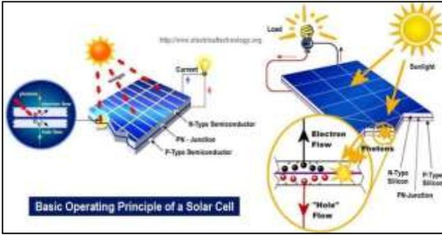
Fig. 2.1: Working of solar cell
