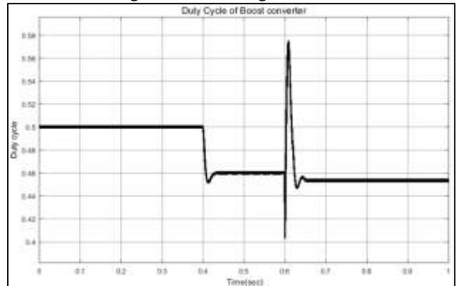
Fig. 6.21: Duty cycle of boost converter
