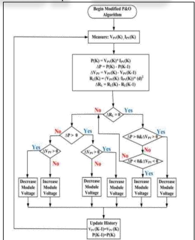
Fig. 6.5: Flowchart of the MPPT algorithm
