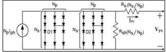
Fig. 6.2: Equivalent circuit model of single-diode for PV array [9]
