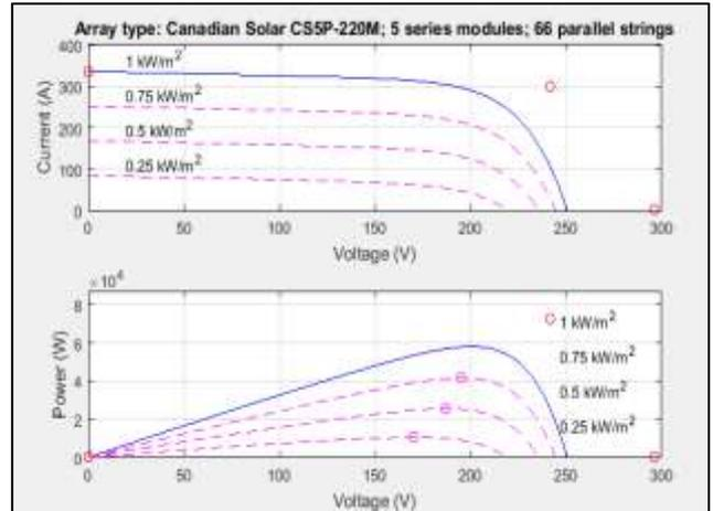
Fig. 6.9: I-V and P-V curve of solar array
