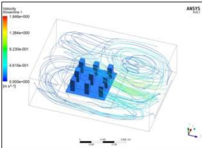
Fig: 5.6. Streamline plot for Rectangular fin
