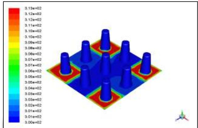
Fig. 8: Temperature Contour of Tapered Fin
