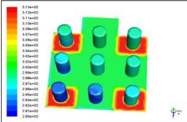
Fig. 9: Temperature Contour of Circular Fin
