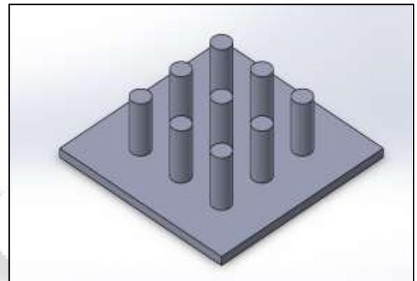
Fig. 3: Cylindrical Fins – Isometric View
