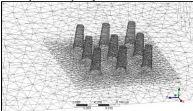
Fig. 7: Meshing – Tapered Fin Wireframe Elements
