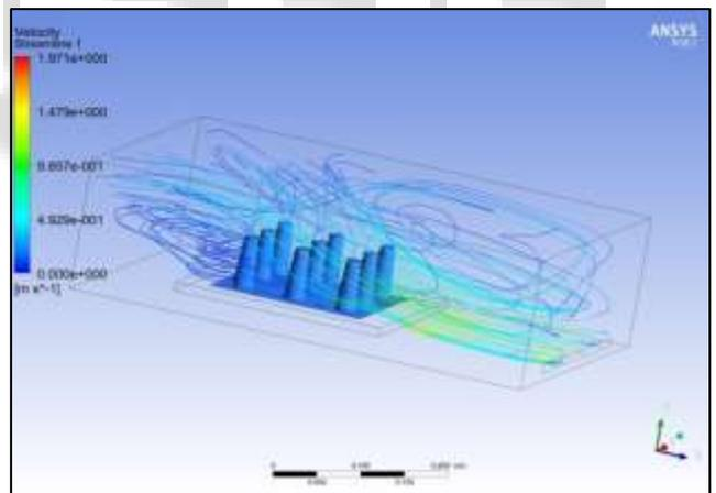
Fig. 5.4: Streamline plot for tapered fin
