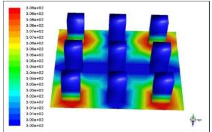
Fig. 10: Temperature Contour of Rectangular Fin
