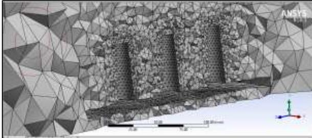
Fig. 6: Meshing – Tapered Fin with Elements
