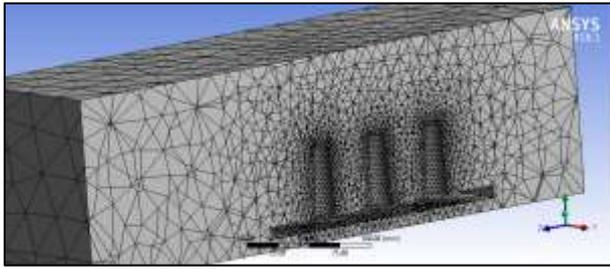
Fig. 5: Meshing – Tapered Fin
