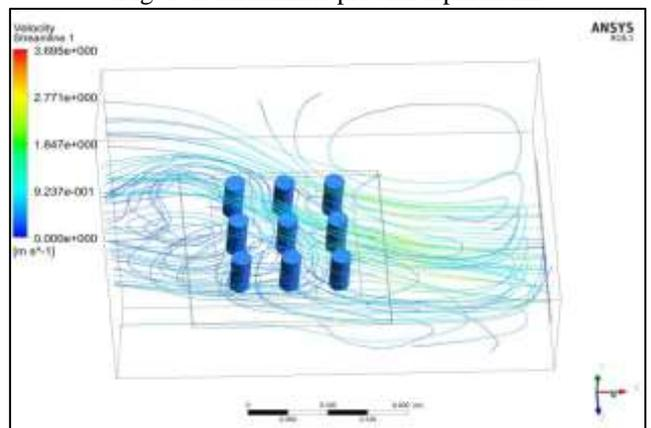
Fig. 5.5. Streamline plot for Circular fin
