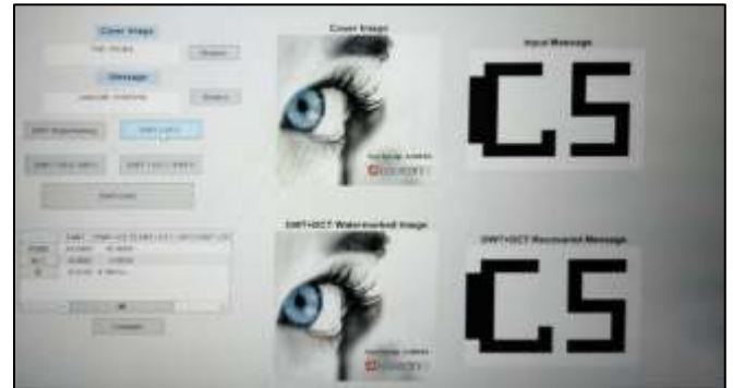
Fig. 3.3: Applying DWT and DCT technique to the input image
