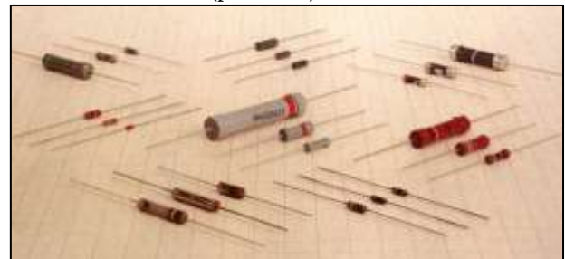
Fig. 4.1: Some low-power resistors
