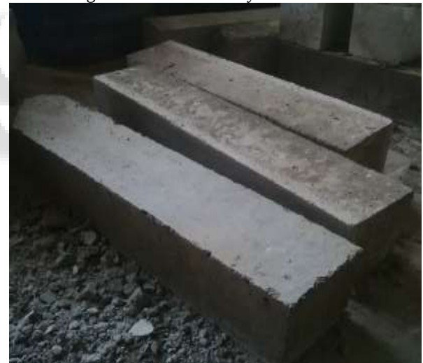
Fig. 3.6: Geo-polymer beam specimen with 5% marble dust
