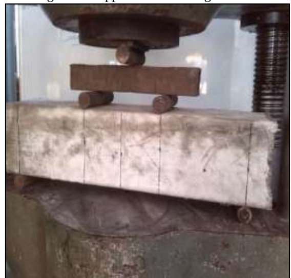
Fig. 15: Ultimate Loading Point of Wrapped Beam
