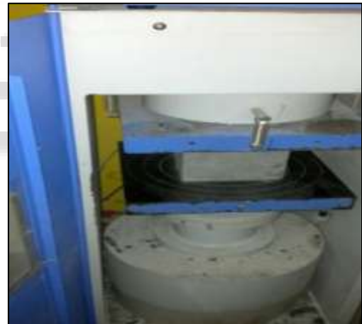
Fig. 5: Concrete Cube Testing In CTM
