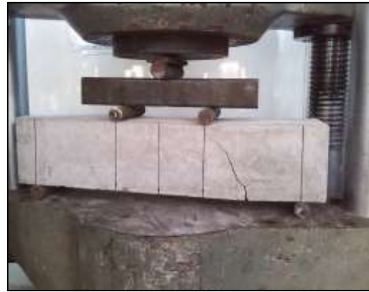
Fig. 9: Cracking of Ordinary R.C.C. Beam in UTM Waste Glass Powder (WGP) With Steel Fibre Reinforced Concrete Beams:
