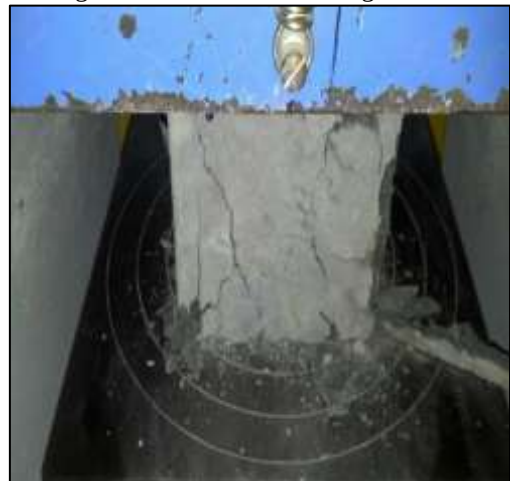
Fig. 6: Concrete Cube at Ultimate Loading Point
