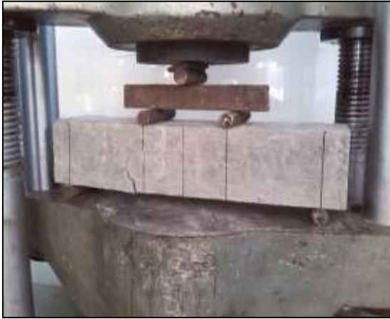
Fig. 11: Ultimate Loading Point of R.C.C Beams WGP with Steel Fibre
