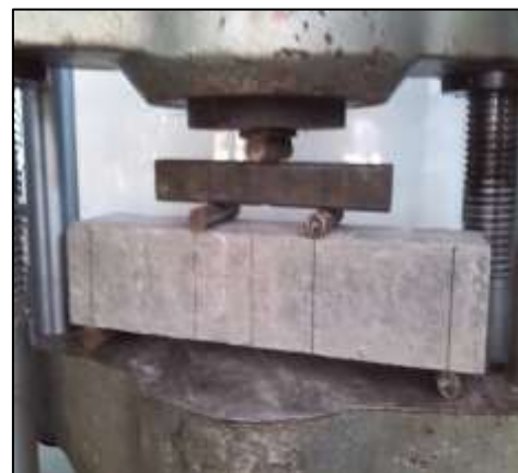
Fig. 16: Testing Of WGP with Steel Fibre R.C.C Beams
