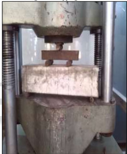
Fig. 14: Wrapped Beam Testing in UTM
