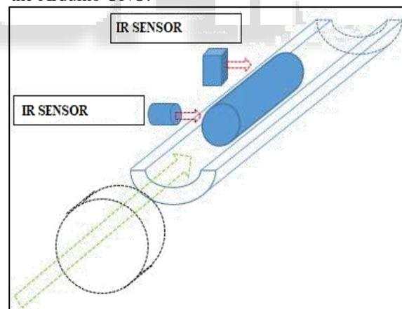
Fig. 3.1: detection of lenth of bottles by IR sensors
