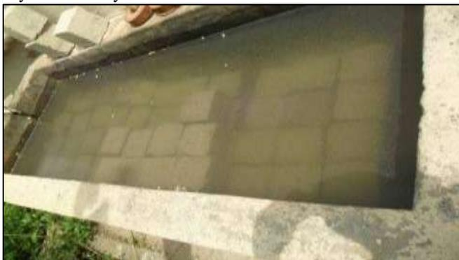
Fig. 3.15.1: Curing of Cubes
