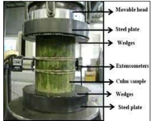
Fig. 1.6.1: Compression Test of bamboo
