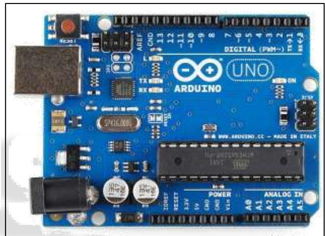
Fig. 4: Arduino board
