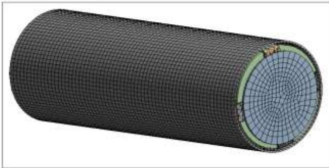
Fig. 16: Meshing H.T plates and thermal jacket with PET water bottle.
