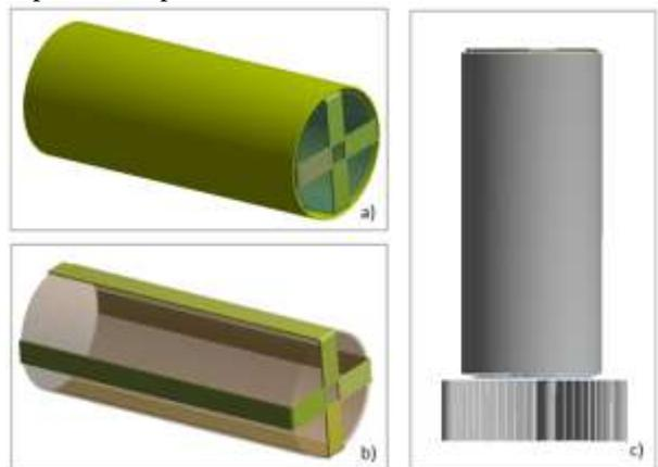
Fig. 15: 3D model of TEC with Al H.T plates and thermal jacket.
