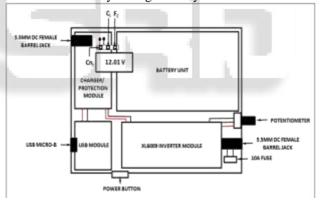
Fig. 9: Block diagram of DC-DC series booster.
