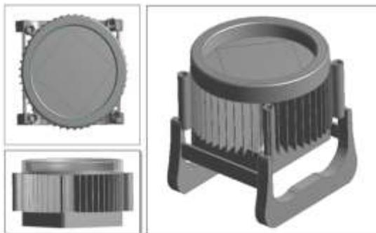
Fig. 13: TEC complete design.
