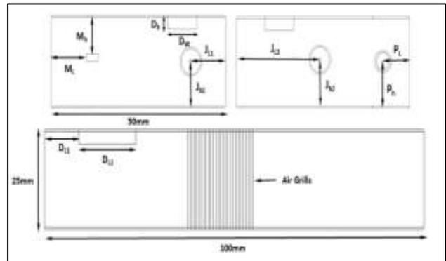
Fig. 8: 2D view of DC-DC series booster.
