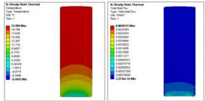
Fig. 17: PET bottle temperature and heat flux simulation (without H.T plates).
