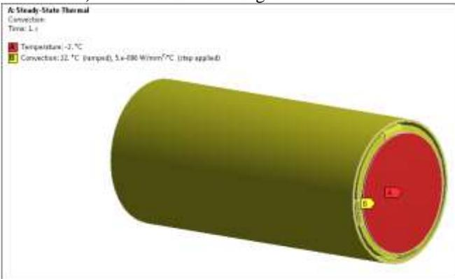
Fig. 17: Boundary conditions of water bottle with H.T plates and thermal jacket.
