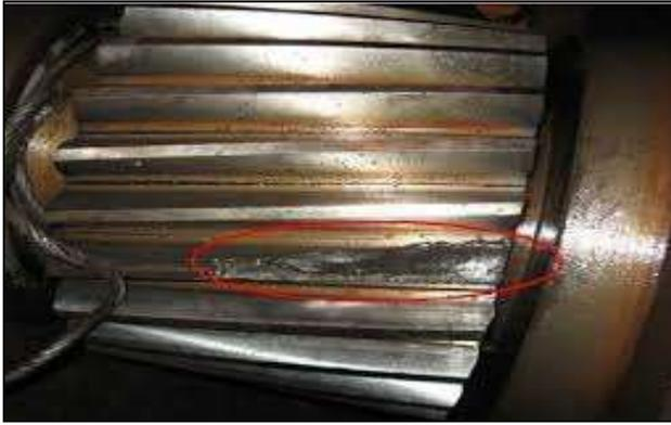
Fig. 3.1: Damaged Helical Gear of Gearbox
