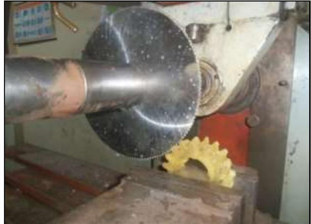
Fig. 5.3: Slicing of a stress frozen photoelastic pinion
