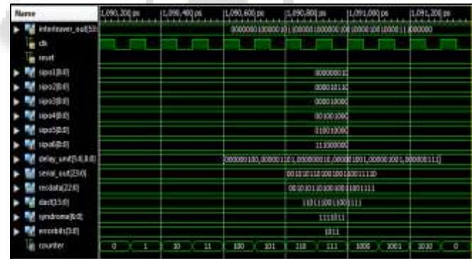
Fig. 6: Simulation result of deinterleaving and decoding – error in 4 data bits
