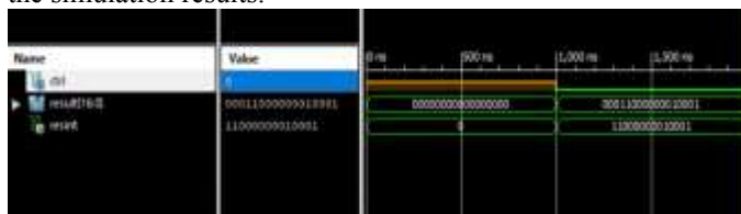
Fig. 1.7: Simulation result of RCM Multiplier Block for the coefficient 12305
