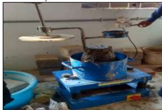
Fig. 4: Vee-bee test on concrete
