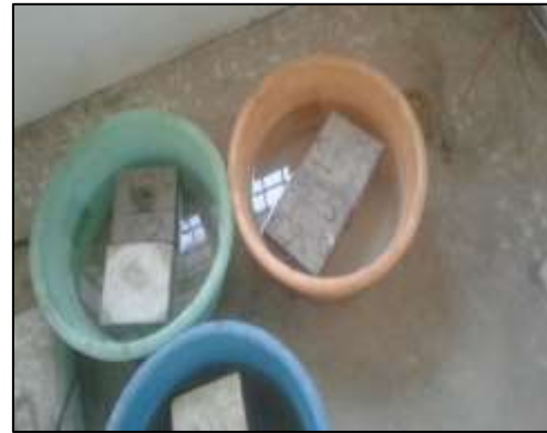
Fig. 2: curing of concrete cubes
