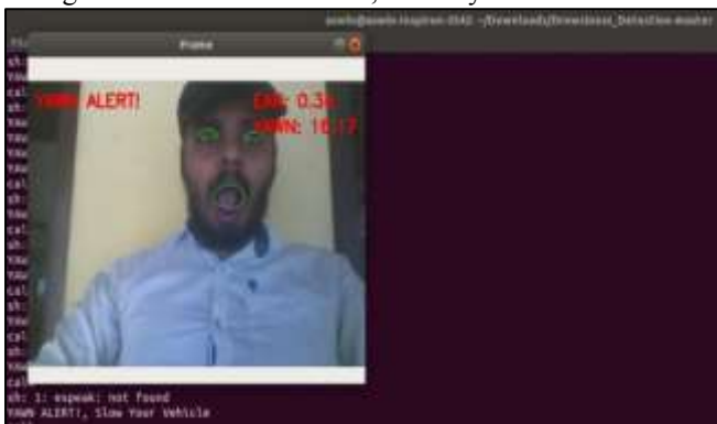
Fig. 6: Yawn Alert, With Eye and Yawn rates.
