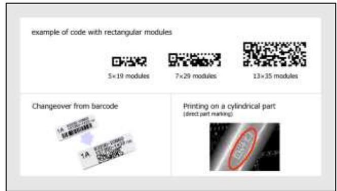
Fig. 3: the rectangular modules of IQR Code
