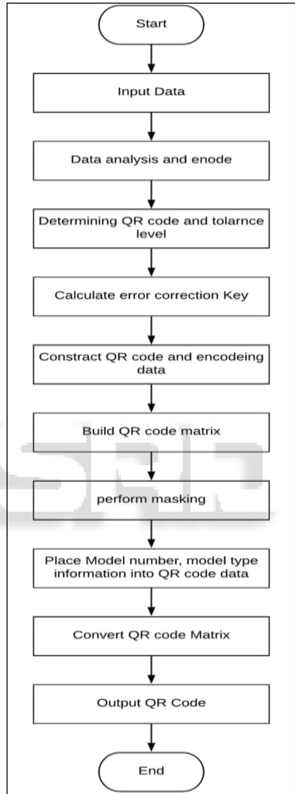
Fig. 12: QR Code encoding process
