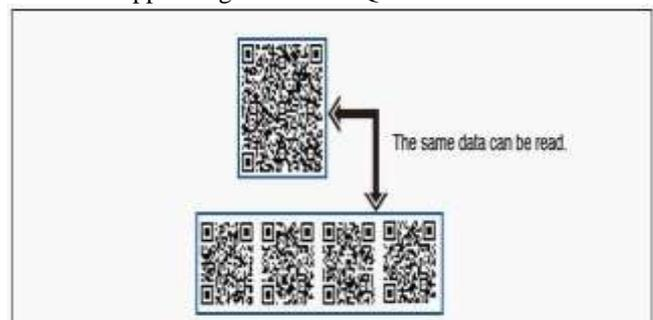
Fig. 1: shows that A QR Code can be divided into more than one QR Code, and all the QR Code also can be stored in one QR Code.
