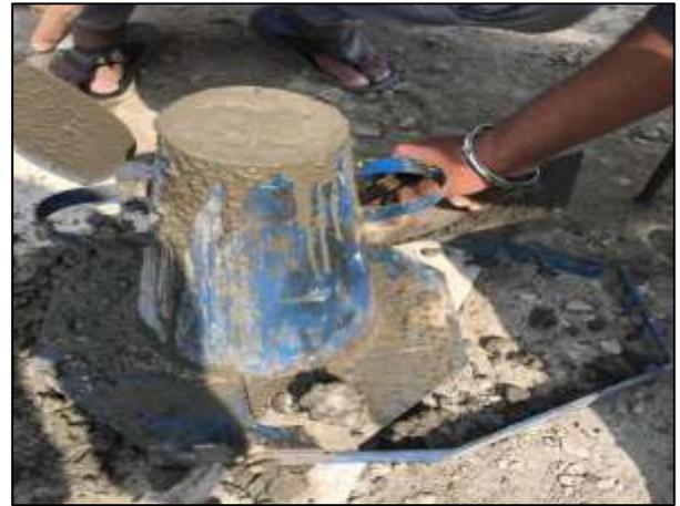
Fig. 6: Workability Test
