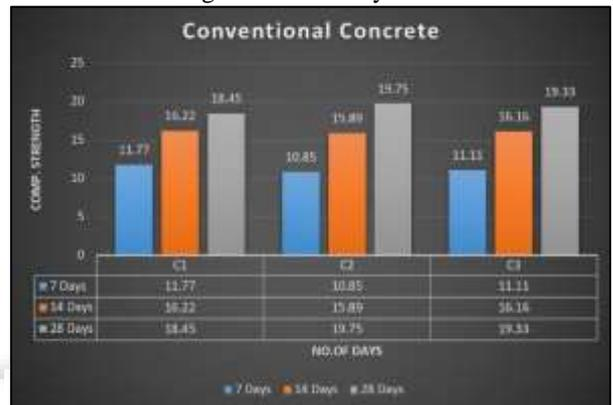
Fig. 7: Compression strength of conventional concrete
