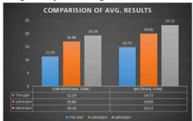
Fig. 9: chart showing comparison between conventional and bacterial concrete
