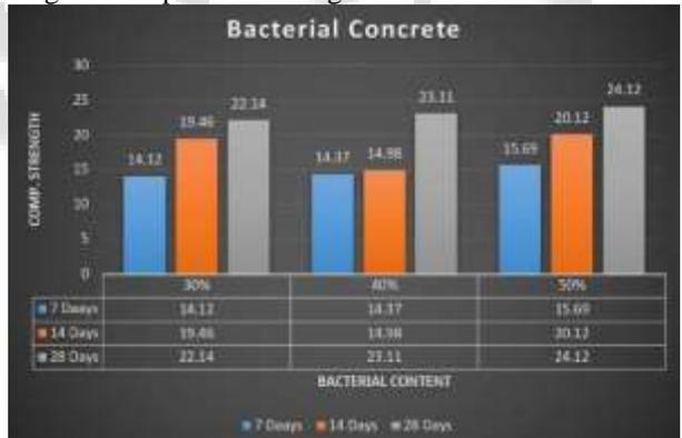
Fig. 8: Compression strength of bacterial concrete.
