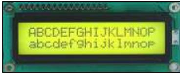
Fig 5: LCD 16\*2 Display Module
