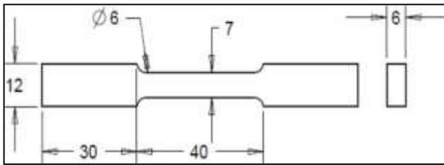
Fig. 5. Tensile test specimen size
