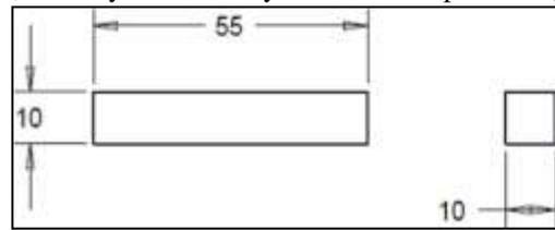
Fig. 7: Impact test specimen size
