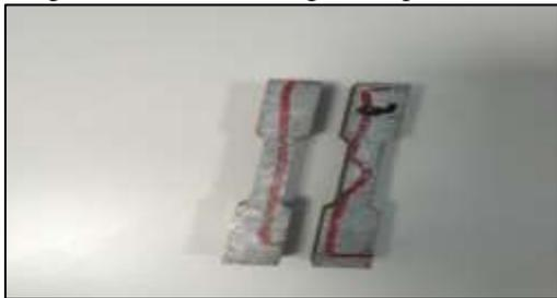
Fig. 6: Tensile test specimen
