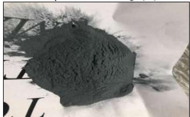
Fig. 1: Coconut shell fly Ash
