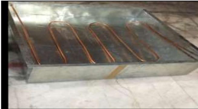
Fig. 1: Experimental setup shows serpentine configuration of pipe
