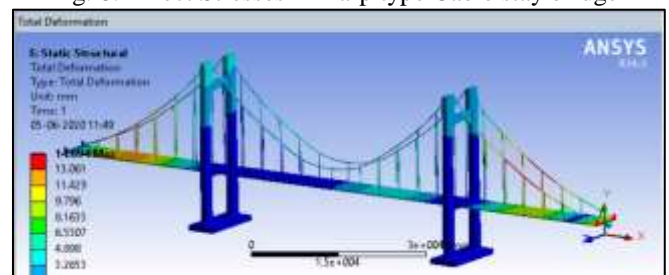
Fig. 9: Total deformations in Suspension type Cable Stay Bridge
