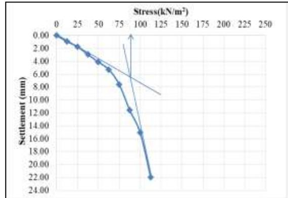
Fig. 4.1: Effect of load intensity on settlement without using waste plastic cups from the 200 mm square plate footing
