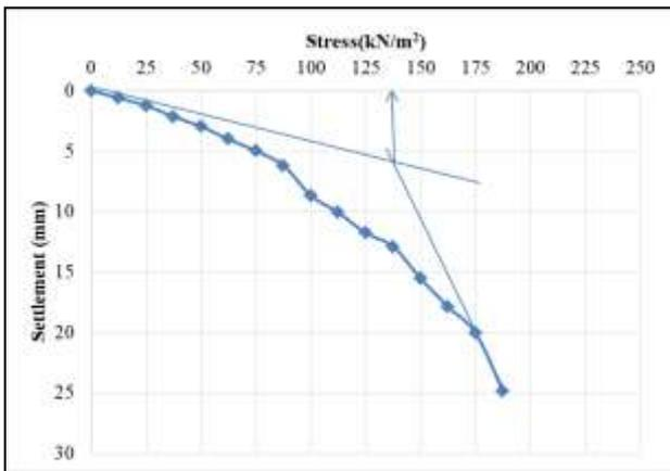
Fig. 4.5: Effect of load intensity on settlement using waste plastic cups at 20 cm depth from the 200 mm square plate footing
