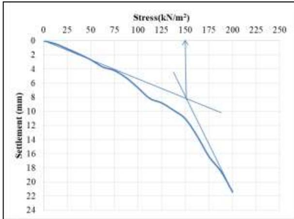
Fig. 4.4: Effect of load intensity on settlement using waste plastic cups at 15 cm depth from the 200 mm square plate footing
