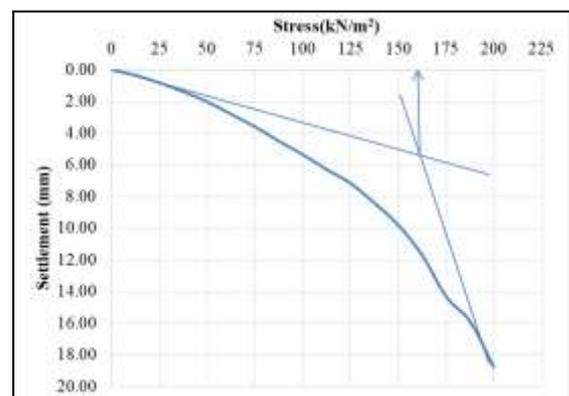
Figure 4.3: Effect of load intensity on settlement using waste plastic cups at 10 cm depth from the 200 mm square plate footing
