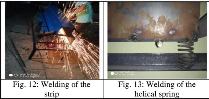
Fig. 12: Welding of the strip
