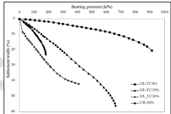
Variation of bearing pressure with footing settlement for G5 with TC 5%, 15% & 30% at ID 80%
