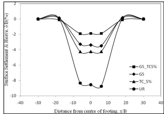
Surface deformation profiles for G5+TC5%, G5, TC5% & UR at bearing stress of 100 kPa, ID 80%
