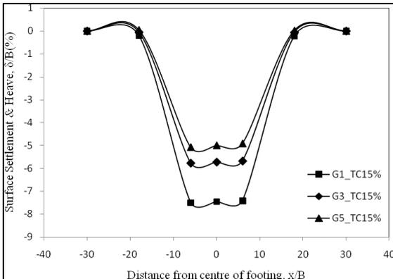
Surface deformation profiles for G1, G3 & G5 +TC15% at bearing stress of 100 kPa, ID 80%
