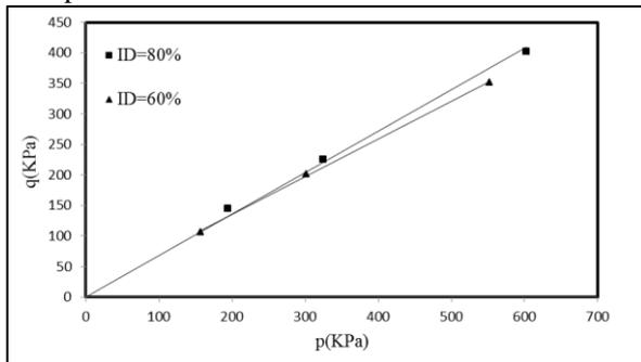
Fig. 3.2: p-q plot for different relative densities of sand under triaxial compression test
