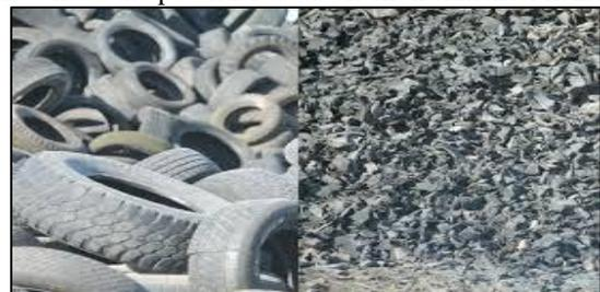
Fig. 1.2: Waste tyres and its shredded form
