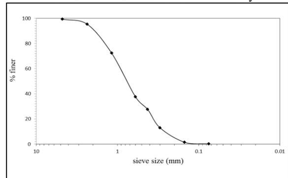
Fig. 3.4: Grain size distribution of tire crumb used in the study
