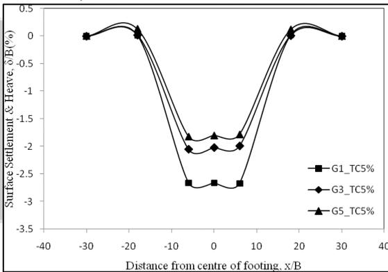
Surface deformation profiles for G1, G3 & G5 +TC5% at bearing stress of 100 kPa, ID 80%
