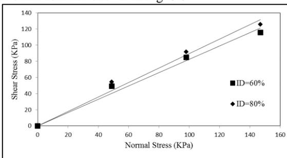
Fig. 3.3 Normal stress-peak shear stress response of sand at different relative densities obtained from direct shear test
