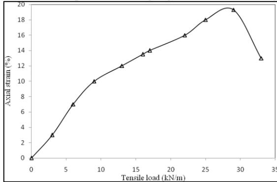
Fig. 3.6: Load-strain behavior of biaxial geogrid used in the study
