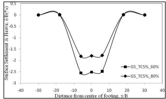
Surface deformation profiles for G5 \_TC5% at bearing stress of 100 kPa, ID 60% & 80%
