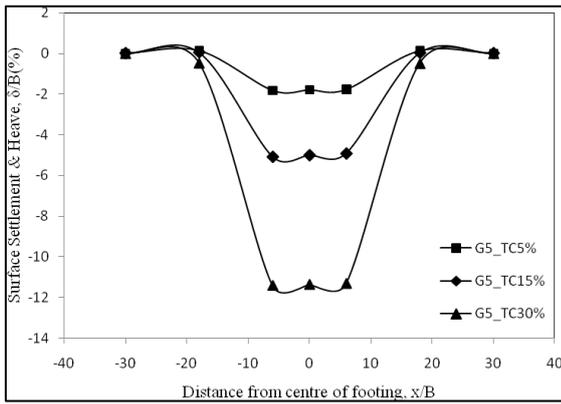
Surface deformation profiles for G5 +TC5, G5+TC15 & G5+TC30% at bearing stress of 100 kPa, ID 80%
