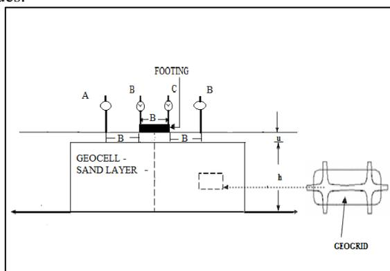
Fig. 3.7: Geometry of the reinforced foundation bed
