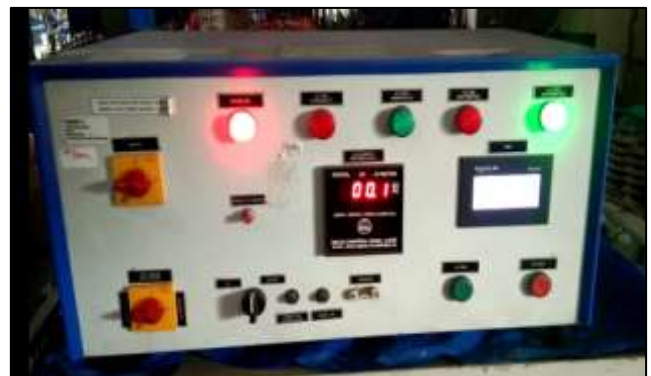
Fig. 7: Breakdown voltage test kit
