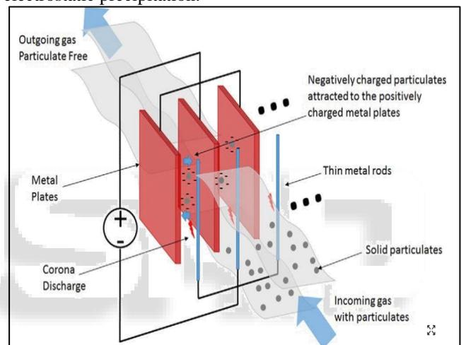
Fig. 1: Principle of Electrostatic Precipitator
