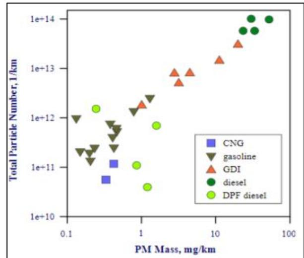
Fig. 2: Particulate matter (PM) emission rate in different fuel engines.
